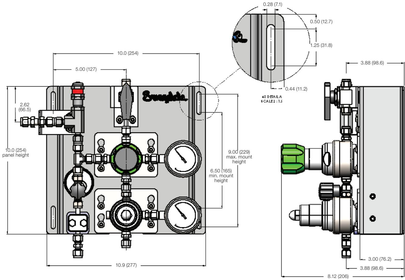
Dual-stage SGP shown. Dimensions are the same for single-stage systems.
