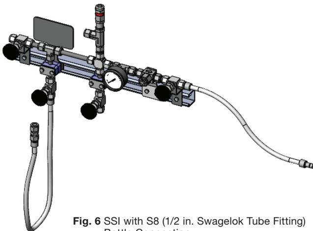
**Fig. 6** SSI with S8 (1/2 in. Swagelok Tube Fitting) Bottle Connection
