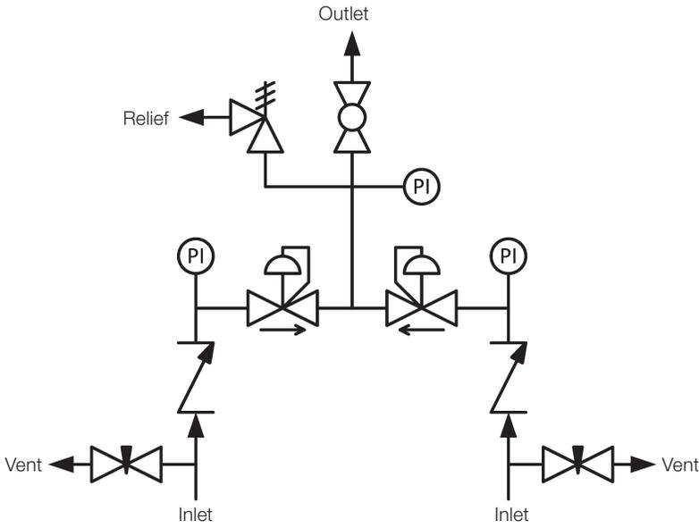
Fig. 19 SCO P&ID without Outlet Pressure Regulator
