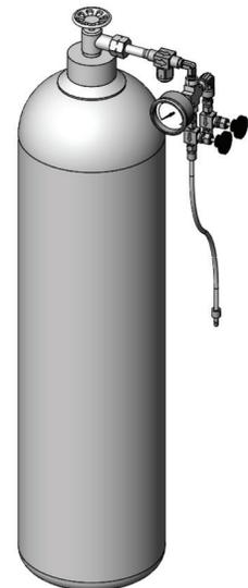
**Fig. 5** SSI for Single Bottle with No Rail
