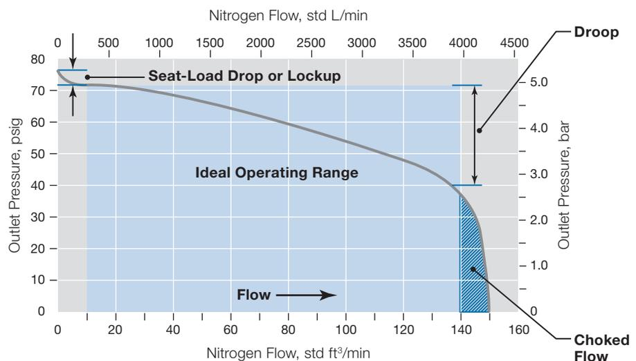
**Fig. 3.** This typical flow curve for a pressure-reducing regulator illustrates several phenomena, including the ideal operating range, droop, choked flow, and seat-load drop or lockup.
