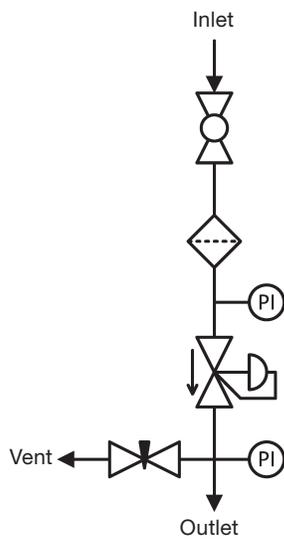
Fig. 17 SPU with Inlet Pressure Gauge and Low-Pressure Vent P&ID
