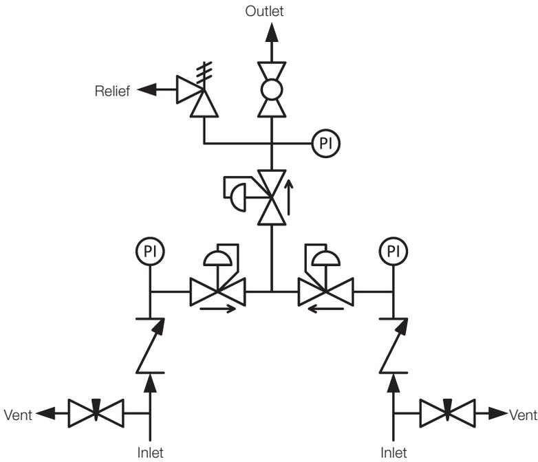
Fig. 20 SCO P&ID with Outlet Pressure Regulator
